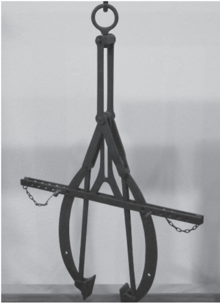
Figure 1.6 Model of an innovative lifting device (17 th century), Modellkammer in the Maximilianmuseum in Augsburg. (Image: Dirk Bühler [44])
