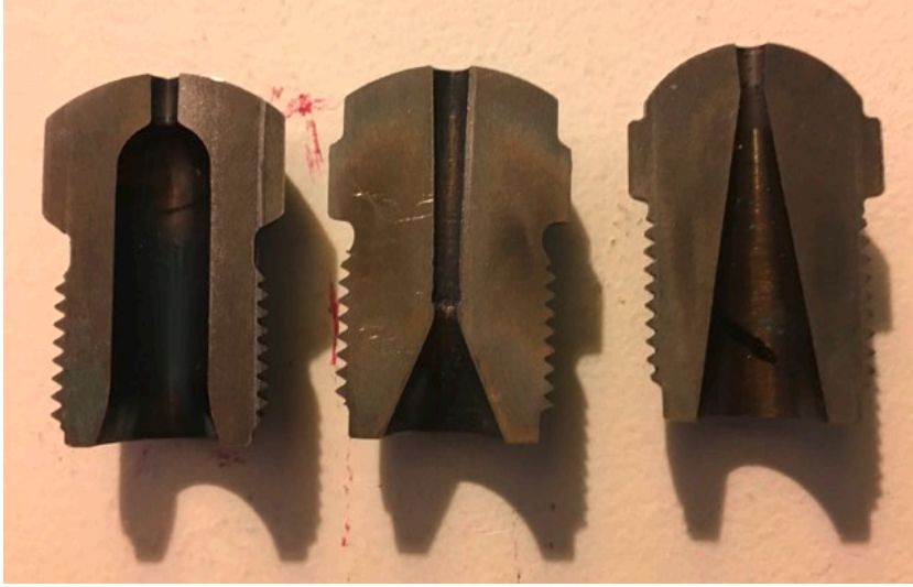
Figure 23.5 Nozzle tips: general purpose, nylon, and full taper
