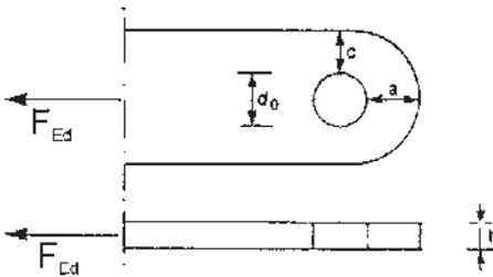
$$\alpha \geq \frac{F_{Ed} \gamma_{M0}}{2t f_y} + \frac{2d_0}{3} ; \quad c \geq \frac{F_{Ed} \gamma_{M0}}{2t f_y} + \frac{d_0}{3}$$
