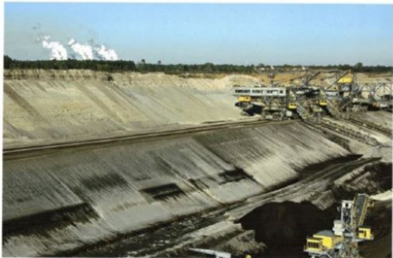
Above: The overburden conveyor bridge F 60 in Lichterfeld near Klettitz. This machine used to remove the spoil or overburden from the top of the coal seam. Since its closure in 1992 it has been an industrial monument and can be visited.
