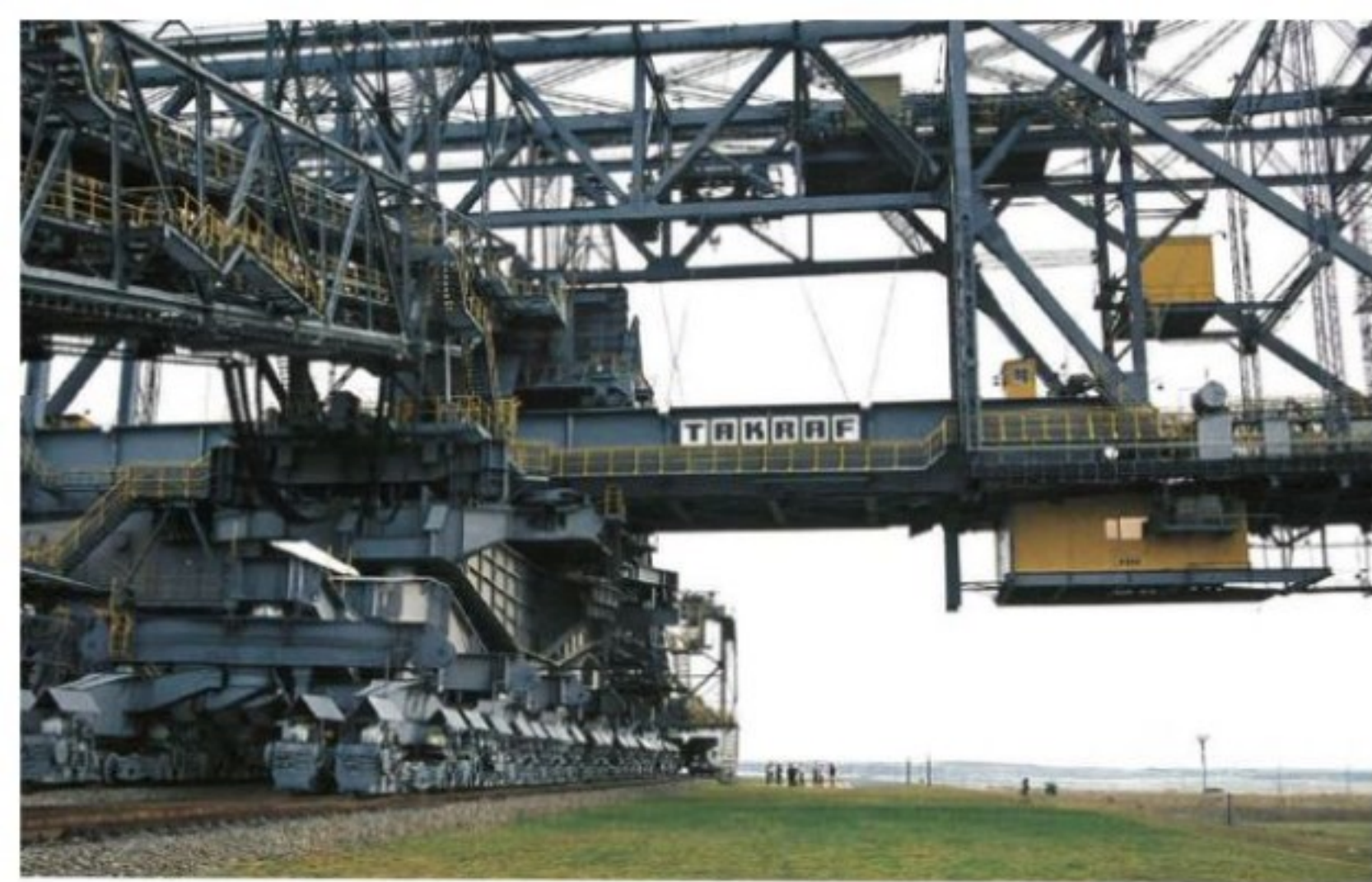
Above: The overburden conveyor bridge F 60 in Lichterfeld near Klettitz. This machine used to remove the spoil or overburden from the top of the coal seam. Since its closure in 1992 it has been an industrial monument and can be visited.
