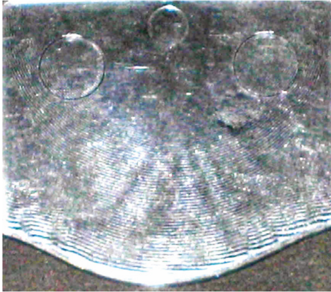
Figure 15.22 Record grooves or orange peel
