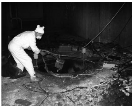
Figure 6.19 Mounting of the aerosol sampling pump in the “Bypass.”
