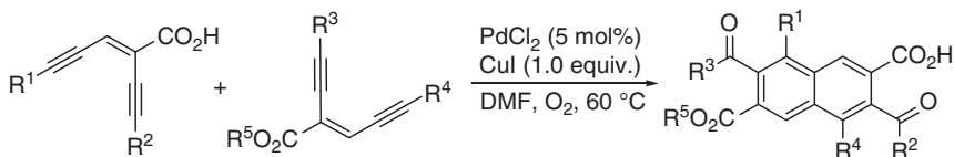
Scheme 1.36 Pd(II)-catalyzed bimolecular carbocyclizations of enediynes to 2,6-diacynaphthalenes.
