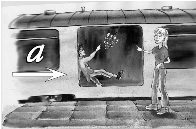
Figure 1.2 A chandelier in an accelerated car. To Alice, the tension force in the deflected chain acquires a horizontal component causing the chandelier to accelerate at the same rate as the car. Tom explains the deflection of the chandelier as the result of the inertial force. This force balances the horizontal component of the chain's tension.
