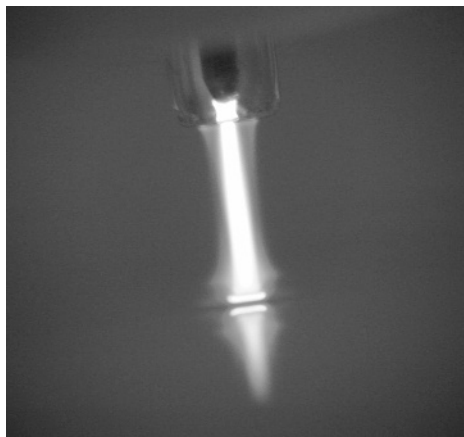
Figure 1.9 RF helium plasma jet hitting a glass substrate. (Source: Photo: Sven Hofman, TU/e.)
