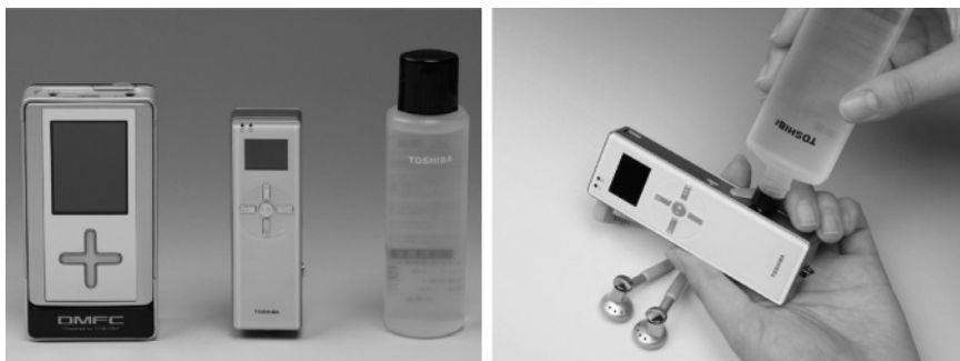
Figure 1.13 TOSHIBA DMFC for portable applications. Direct methanol fuel cell combined with a small backup Li-ion battery. Source: Han 2002 [32]. Reproduced with permission of Elsevier.
