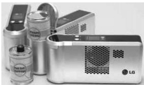
Figure 1.14 The 25 W DMFC prototype to power laptop computers, by LG Chemical in 2005. Source: Li 2013 [26]. Reproduced with permission of Elsevier.
