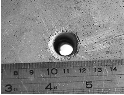
Figure 1.9 A 12 mm diameter, 10 cm deep hole in a concrete slab produced by a microwave drill that was mechanically assisted for debris removal. Courtesy Eli Jerby, Tel Aviv University, Ramat Aviv, Israel.
