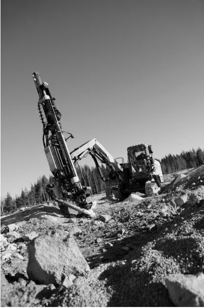
Figure 1.15 Atlas Copco SmartRig ROC D9C. The drill literally drills by itself. Courtesy Atlas Copco Rock Drills AB, Sweden.
