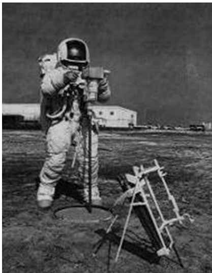
Figure 1.17 Apollo lunar surface drill being tested at the Kennedy Space Center. The handle, battery, power head and drill stems are visible. The drill stem rack is in the foreground with a set of stem sections and a wrench on the right. Courtesy NASA (photograph S70-29673).
