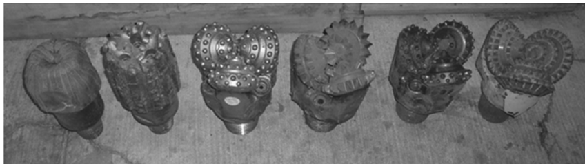
Figure 1.16 Petroleum drill bits are produced in various shapes depending on the formation that needs to be penetrated.
