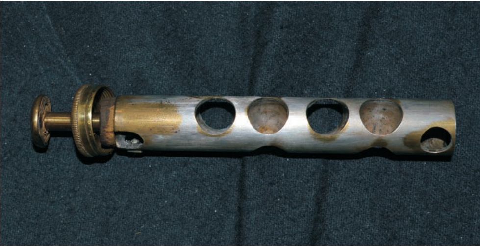
FIGURE 3 Dual airflow valve, cor Sax à 6 pistons, serial number 37403, Brussels MIM inventory number 3167.
