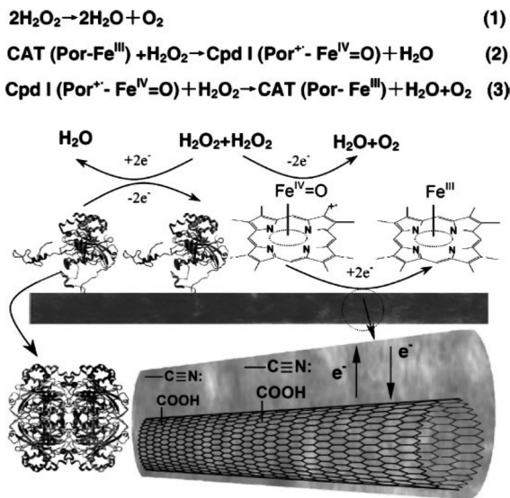
Fig. 1.16 Schematic representation of the nanofibrous poly(acrylonitrile- co -acrylic acid) membrane containing MWCNTs, as well as the promoted electron transfer from hydrogen peroxide to the immobilized catalase through the PANCAA/MWCNTs nanofiber. Reprinted from [209] (reproduced by permission of Wiley-VCH).
