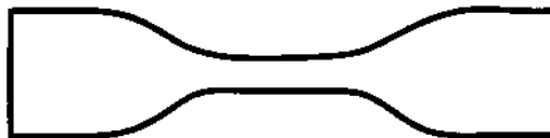
Figure 3.2 Rubber dumbbell test specimen.
