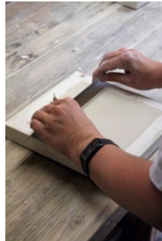
d) Excess material protruding above upper edge of mold is scraped off
