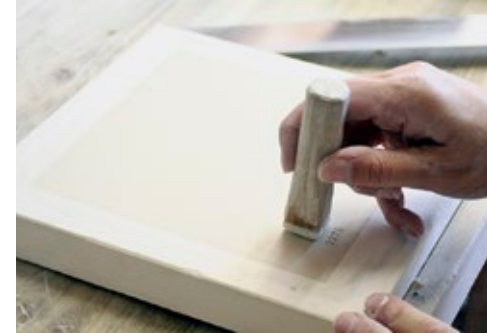
e) Factory mark and plaque number stamped into rear surface
