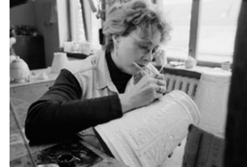
f) Lampshade is touched up prior to firing
