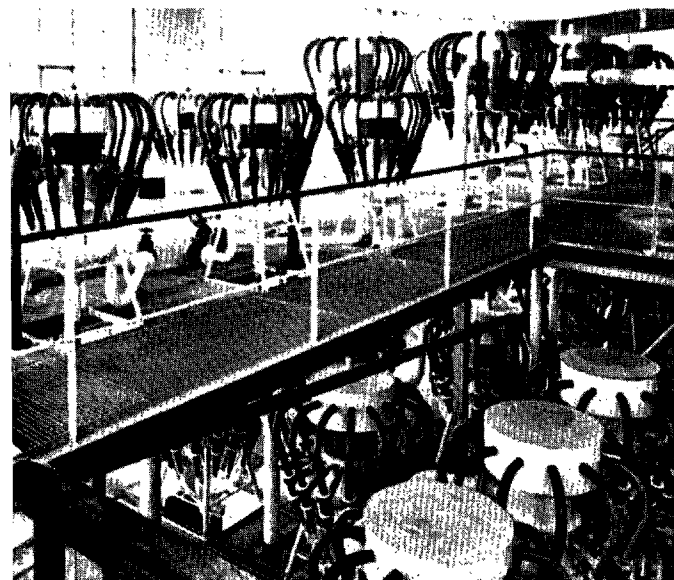
Amberger Kaolinwerke cyclone plant beneficiates kaolin, making selective classifications on the basis of particle size.
