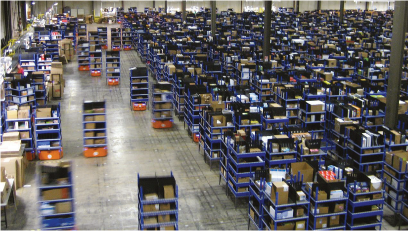
Figure 1.1: Grid-flow with transport vehicles. Photograph of Amazon Kiva Systems [21]
