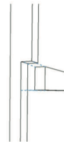
Figure 5.24: Examples of wood joints from the house in Arnavutköy
