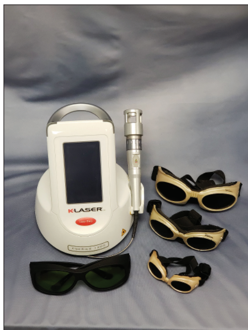
Figure 1.10 A class IV veterinary therapeutic laser with human and animal personal protective eyewear. Source: Lisa P. McFaddin.
