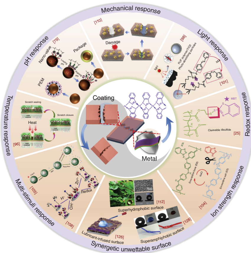
Figure 1.5 Release of corrosion inhibitors from containers in response to different stimuli. Source: Fu et al. [80]/with permission of Elsevier.
