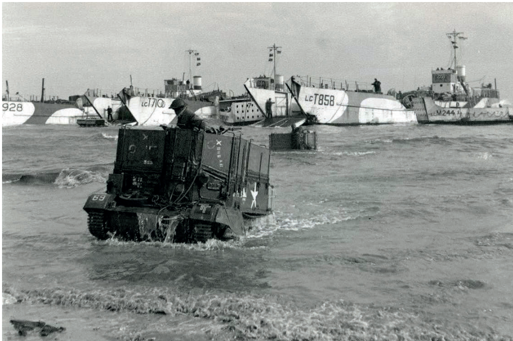
...We had... been waterproofing the carriers... (waterproofed carriers, D-Day) - IWM B5244
