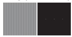
being two pixels wide. The image on the right is the Fourier spectrum of the image on the left, showing the dc term and the frequency terms corresponding to the stripes. (Remember, the spectrum is symmetric so all components, other than the dc term, appear in two symmetric locations.)
