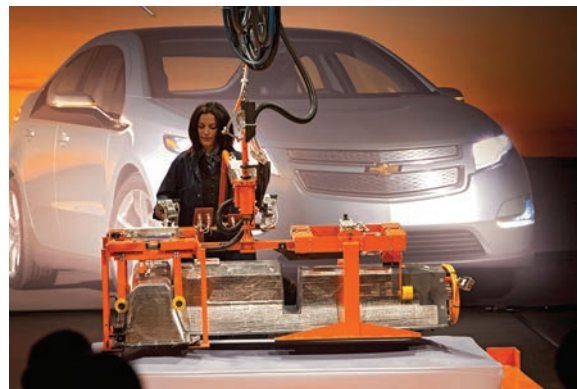
A lithium-ion battery pack for General Motors' electric vehicle, the Chevrolet Volt, which has been on the market since 2011.
