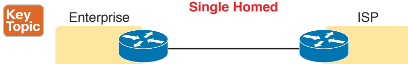
Figure 12-4 Single-Homed Design: Single Link, One Home (ISP)
