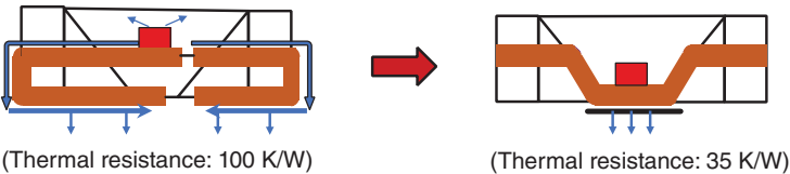
Figure 1.10 Mid-power LED PLCC package thermal management design evolution.
