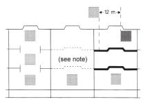
**Note:** One of the two decks must be resistant to fire and to liquid.
