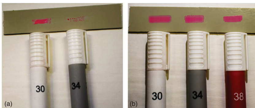
Figure 1.16 Dyne pen application on a polymeric non-treated (a) and plasma-treated (b) adherend.
