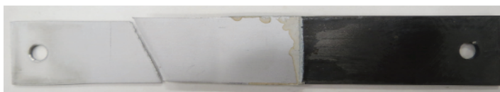
Figure 1.33 Adhesive joint with adherend failure.
