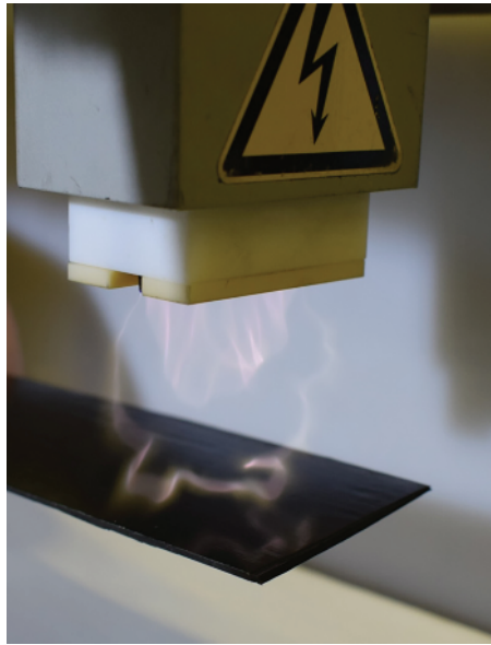
Figure 1.14 Surface of the polymeric material to be treated with plasma.
