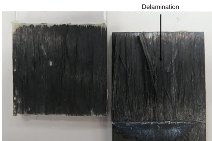
Figure 1.36 Example of delamination failure of composite joints.
