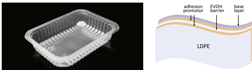
Figure 1.6 Multilayer packaging: transparent and tough, barrier against oxygen and water, thermoformable, and lightweight. Allows safe storage of food [5] (Picture source: nikkytok/Shutterstock-com (left) and INEOS Styrolution (right))
