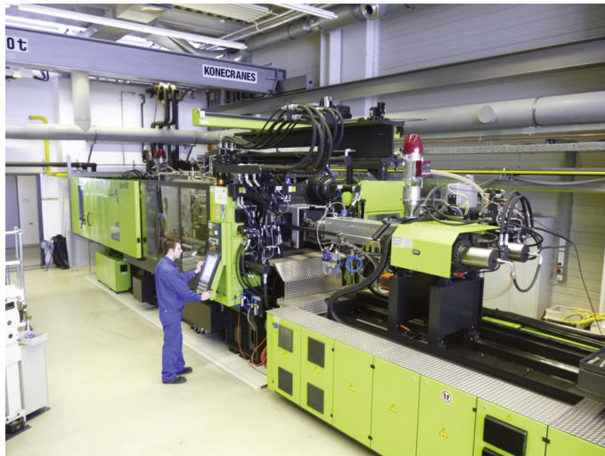
Figure 1.8 Advanced injection molding machine, allowing addition of gases and co-injection of different thermoplastics (courtesy of Neue Materialien Bayreuth GmbH)
