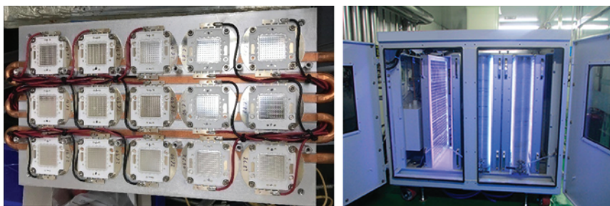
Figure 1.10 Examples of large-scale photoreactors built by Merck (left) and Amgen (right).
