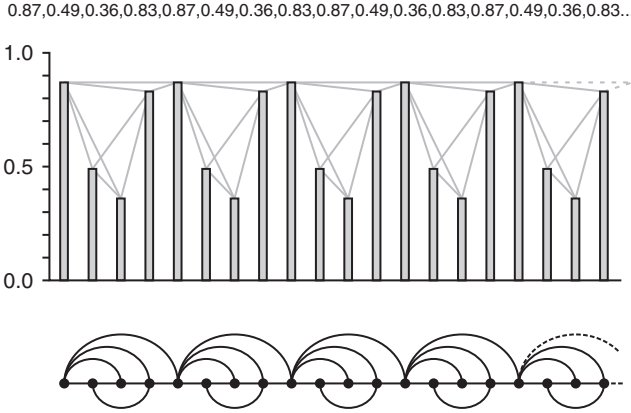
Figure 1.1 Illustrative example of the natural visibility algorithm. In the upper part, we plot a periodic time series and in the bottom part, we represent the graph generated through the natural visibility algorithm. Each datum in the series corresponds to a node in the graph, such that two nodes are connected if their corresponding data heights fulfill the visibility criterion of equation 1.1.
