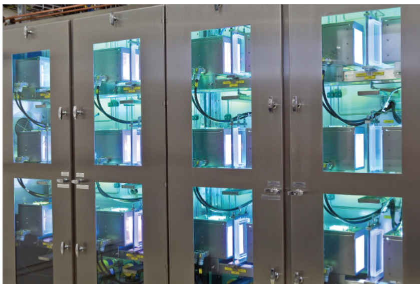
Figure 1.6 Flow photochemical production plant. (Oelgemöller 2012 [76]. Reproduced with permission of Wiley.)
