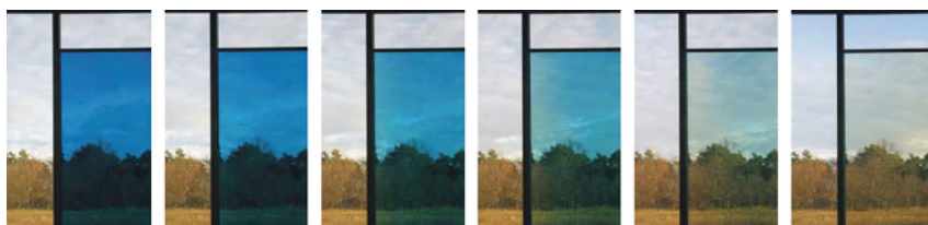
Figure 1.4 Switching sequence of an electrochromic laminated glass. Source: Baetens et al. 2010 [28]. Reproduced with permission of Elsevier.
