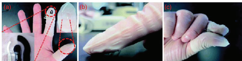
Figure 1.3 Schematic delineating voltammetry of microparticles on a wearable Forensic Finger . (a) The Forensic Finger shows the three electrode surfaces screen-printed onto a flexible nitrile finger cot (bottom left inset), as well as a solid, conductive ionogel immobilized on a similar substrate (top right inset). (b) "Swipe" method of sampling to
