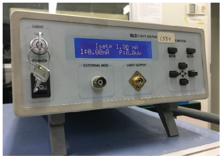
Figure 1.4 Photo of a benchtop SLD light source. Source: Junferg Jiang.
