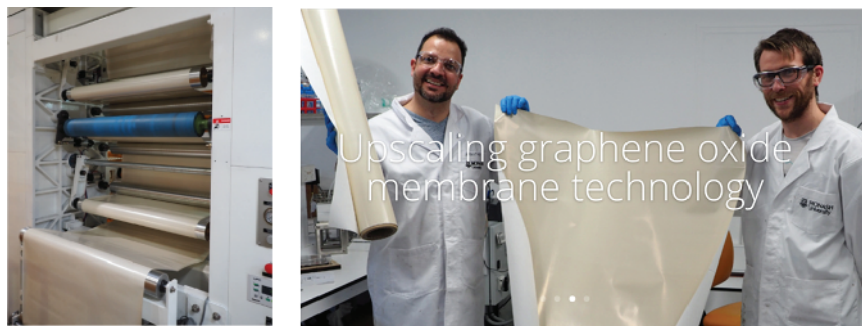
Figure 1.20 Photos showing industrial-scale production of GO membranes in Melbourne, Australia, developed by Monash University and Ionic Industries. Source: https://www.monash.edu/engineering/about-us/news-events/latest-news/articles/2018/monash-pours-energy-into-clean-water-future . Reproduced with permission.
