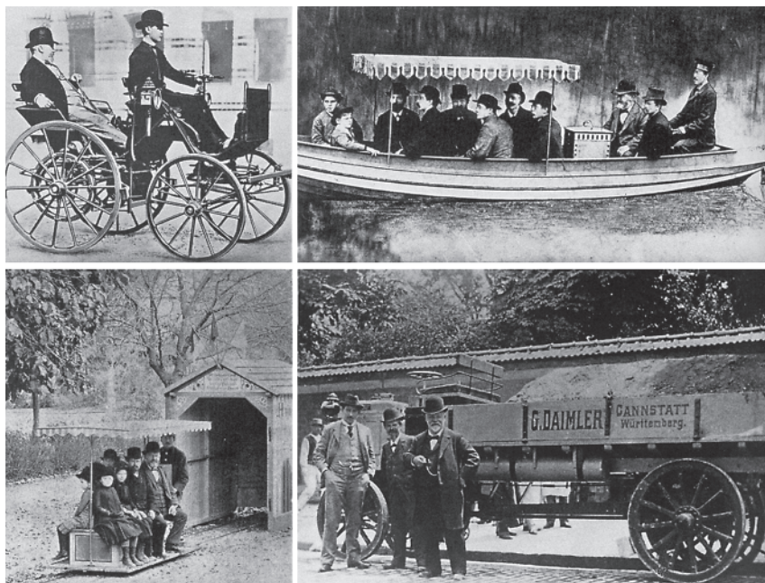
Figure 1.3 Daimlers “small, lightweight, high-speed engine” powering the first four-wheeled passenger car, “the motor carriage” from 1886; a boat (1886); a fair train (1887); a truck (1889).
